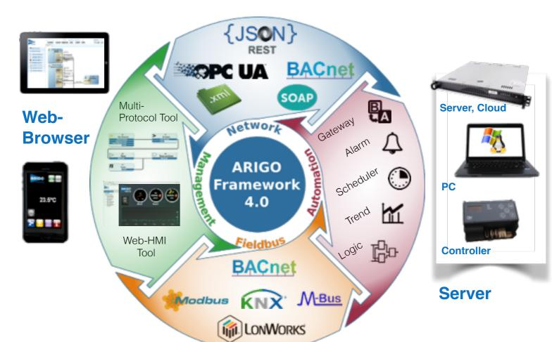
The ARIGO Framework 4.0 is a Web-Service that runs on an embedded Controller, PC or an enterprise system. It provides a Multi-Protocol Network Management Tool for BACnet, M-Bus, LON, Modbus and others. This allows to manage devices from different manufacturers and protocols to be installed and combined in a simple, intuitive way.
